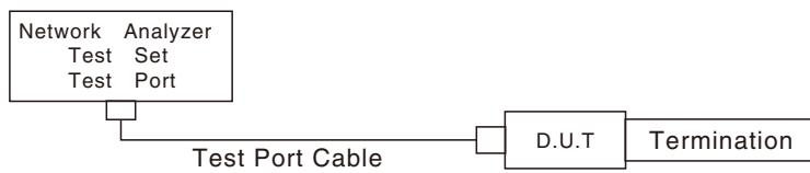
Note 1: Cable type connectors were measured with SMA conversion adapters attached to both ends of the harness product of a suitable 100 cm cable.
