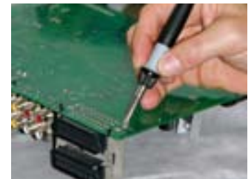
High-mass through-hole soldering with the i-Tool
