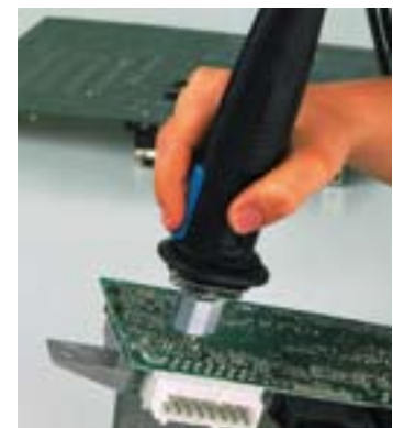
High-mass through-hole desoldering
