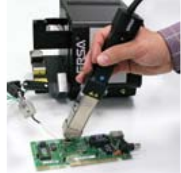
Rapid, simple and safe hand-held component removal
