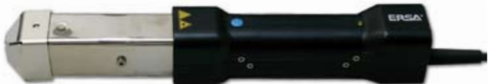
ERSA Hybrid Tool with 200 W heating power and positioning laser (class II) in the handle, weight 300 g
