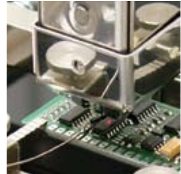
Temperature-controlled SMD soldering
