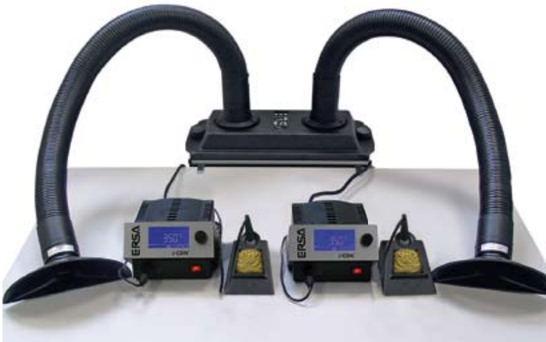
i -CON C soldering stations with EA 110 plus i solder fume extraction: intelligent filter unit control by means of soldering stations' STANDBY function - filter unit is started as soon as one of the soldering stations is operated
