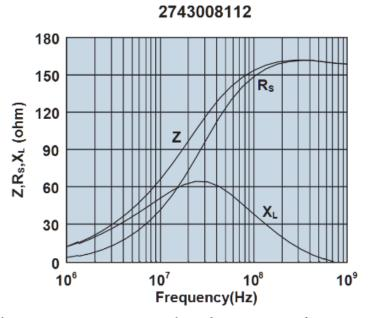
Impedance, reactance, and resistance vs. frequency.
