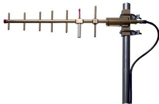
1-port sector (yagi) antenna, 806–869 MHz, 60° HPBW, fixed electrical tilt. Mounting pipe diameter, max. 3".
