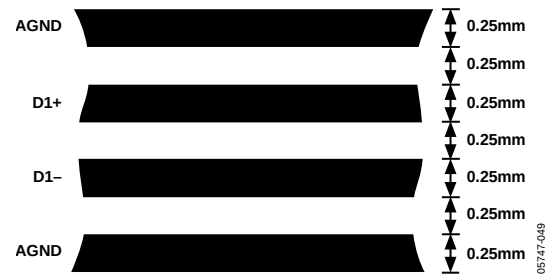
Figure 61. Arrangement of Signal Tracks
