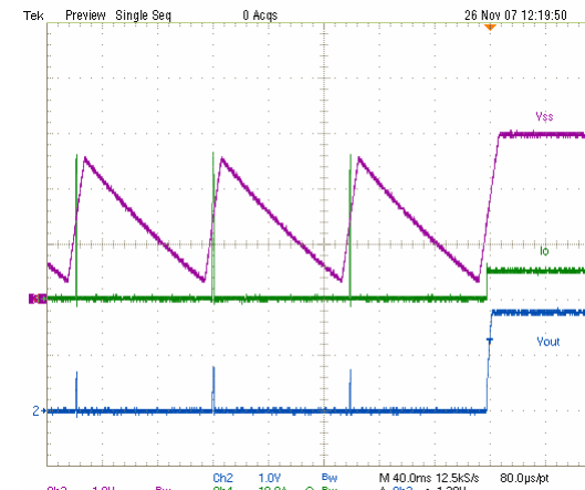
Fig. 9 Shorted Hiccup Condition Recovery
