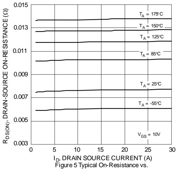
Figure 5 Typical On-Resistance vs.
