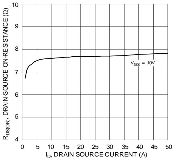
Figure 3 Typical On-Resistance vs.
