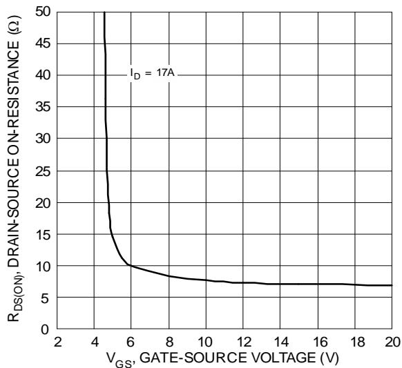
Figure 4 Typical Drain-Source On-Resistance
