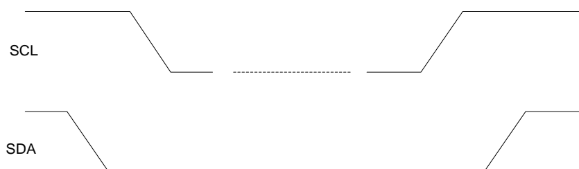
Figure 23: I 2 C START and STOP Conditions
