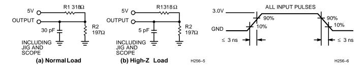
THÉVENIN EQUIVALENT Equivalent to:  $121\Omega$ OUTPUT Q **-**O 1.91V
