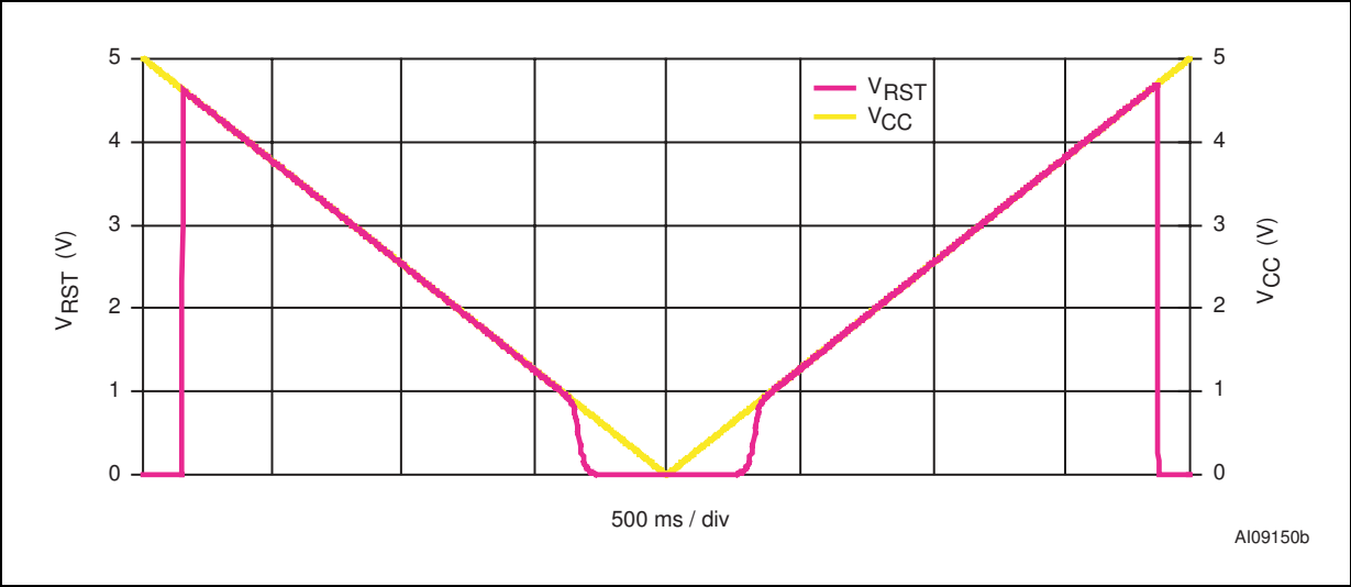
Figure 29. RST output voltage vs. supply voltage
