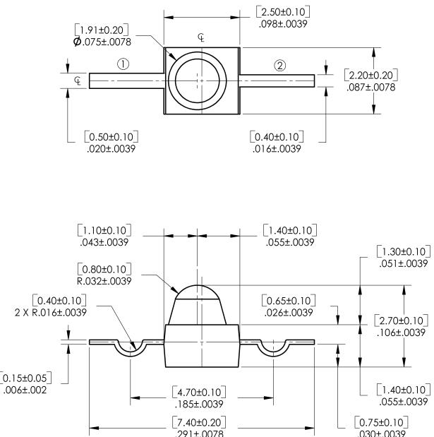
DIMENSIONS ARE IN INCHES AND [MILLIMETERS].
