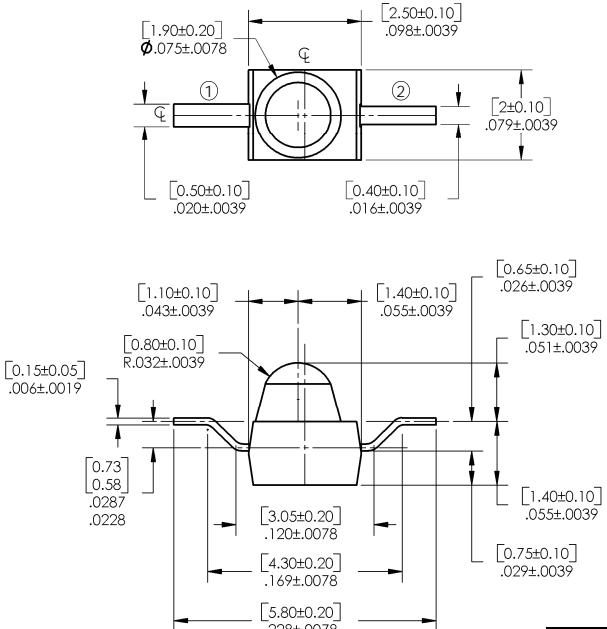
DIMENSIONS ARE IN INCHES AND [MILLIMETERS].
