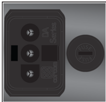
Figure 4-8 SYS-350 DC Power Interface
