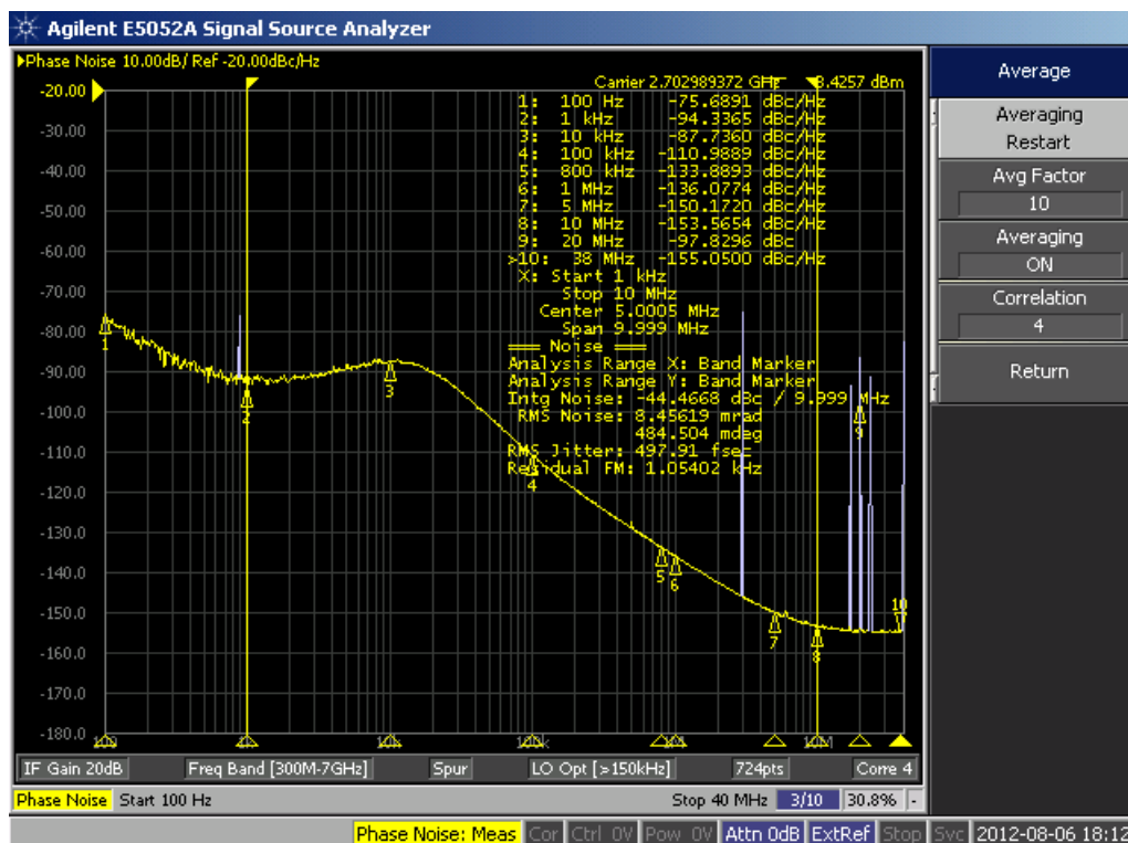
Figure 36. Fvco = 2703 MHz (No Divide)
