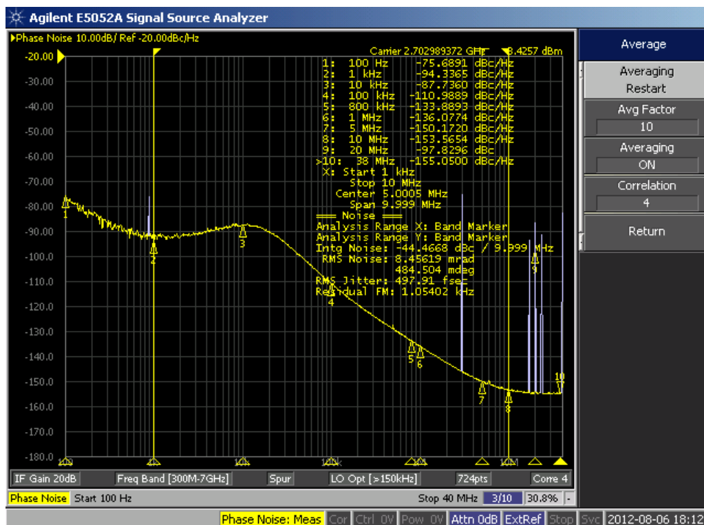
Figure 38. Fvco = 3403 MHz (No Divide)
