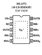
\*THERMAL PAD MUST BE CONNECTED TO NEGATIVE SUPPLY: V<sub>S-</sub>.
