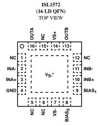
\*THERMAL PAD MUST BE CONNECTED TO NEGATIVE SUPPLY:  $V_{S}$ .. QFN PACKAGE CAN BE USED IN SINGLE AND DUAL SUPPLY APPLICATIONS.
