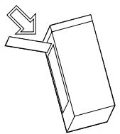
5. Place the new battery in the UPS. Use care to avoid pinching the wires.
