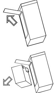
1. Lay the UPS on its left side. Remove the two screws holding on the battery door and open the door.
