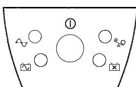
With the UPS plugged in, press and release the On/Off/Test button to supply power to the loads.
