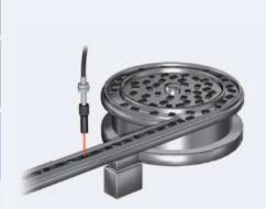
· Small-spot is ideal for detecting minute objects. Select the Fiber Unit that is best suited for the workpiece size and installation distance.
