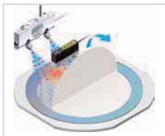
Measuring surface potential when removing BG sheets
