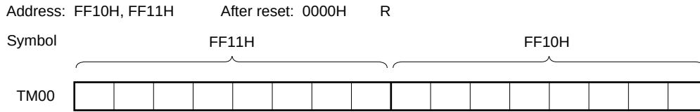
Figure 6-2. Format of 16-Bit Timer Counter 00 (TM00)
