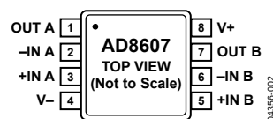
Figure 2. 8-Lead MSOP (RM Suffix)
