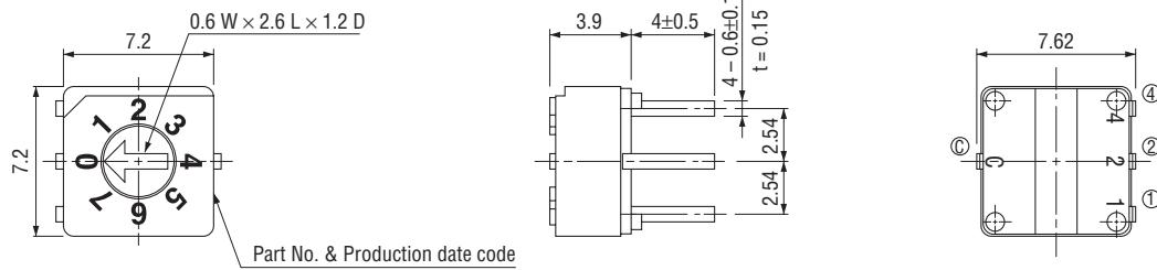
Unless otherwise specified, tolerance:  $\pm 0.3$  (Unit: mm)
