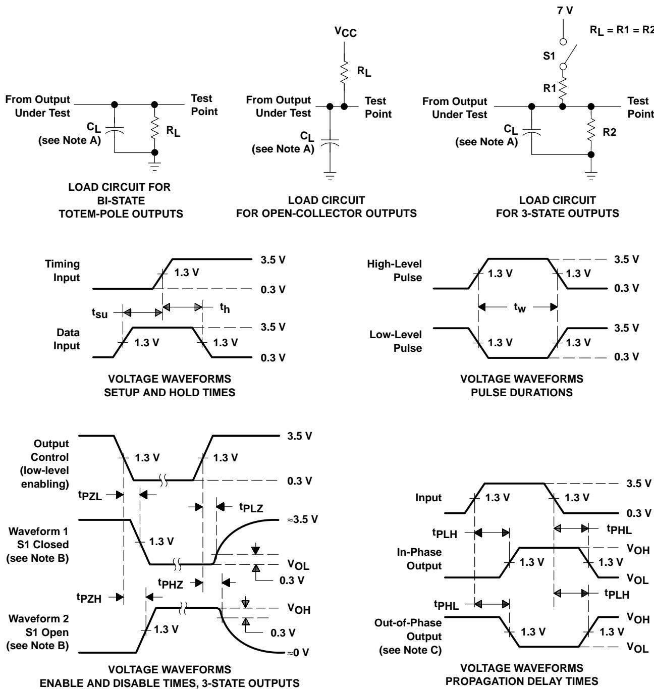
Figure 1. Load Circuits and Voltage Waveforms
