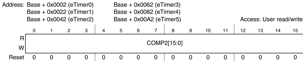
Figure 26-4. Compare register 2 (COMP2)
