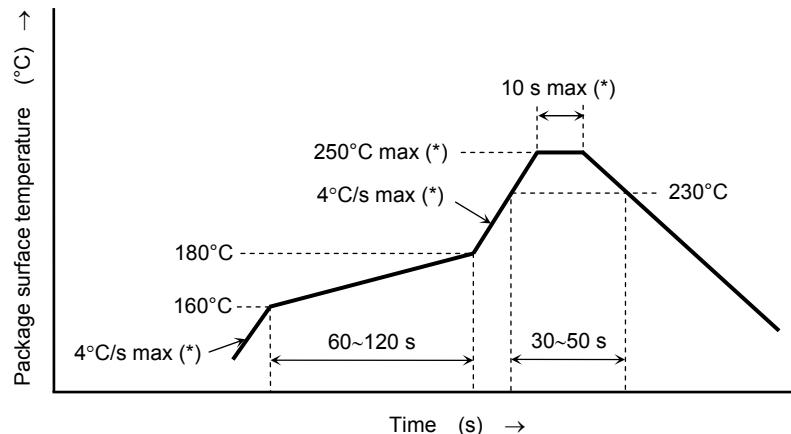
(\*)The product is evaluated using above reflow soldering conditions. No additional test is performed exceed the condition (i.e. the condition more than MAX values) as an evaluation.
