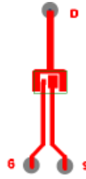
⑧ Mounted on minimum footprint full size board with metalized back and with small clip heatsink (still air)
