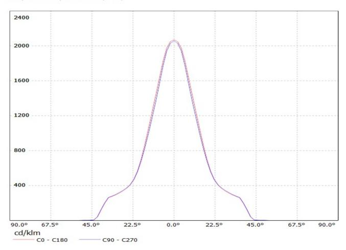
Luminaire: Ledil Oy C11773\_Venla-S-Vega C11773\_Venla-S-Vega Lamps: 1 x Philips Luxeon S (warm) 560,4lm @ 250mA
