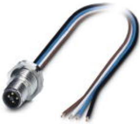
Flush-type connector, Power, 4-position, Plug, M12, T power, Rear mounting, M16 x 1.5, Individual wires, cable length: 0.5 m
