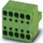
PCB connector, nominal current: 41 A, rated voltage (III/2): 1000 V, nominal cross section: 6 mm<sup>2</sup>, number of positions: 12, pitch: 7.62 mm, connection method: Push-in spring connection, color: green, contact surface: Tin
