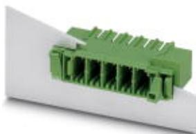
Feed-through header, nominal current: 41 A, rated voltage (III/2): 630 V, nominal cross section: 6 mm<sup>2</sup>, number of positions: 12, pitch: 7.62 mm, color: green, contact surface: Tin, mounting: Wave soldering, pin layout: Linear pinning, solder pin [P]: 4.9 mm
