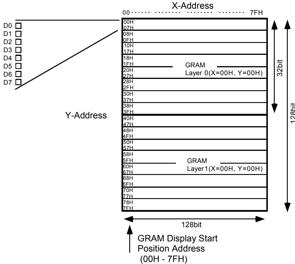
This module has 2 layers - Layer 0 and Layer 1. Each layer in this display consists of 128 by 64 dots. Display merging using these 2 layers can be done with the Display ON/OFF command. Refer to 9.2 on page # 8 for details.
