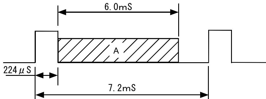
An FRP signal is triggered each time the display is refreshed by the module from its own memory. Smooth scrolling can be achieved by synchronizing the change of display start address with the FRP signal from module. The area marked as "A" is optimal for writing commands.
