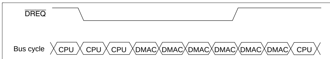
Figure 11.13 DMA Transfer Example in the Burst Mode
