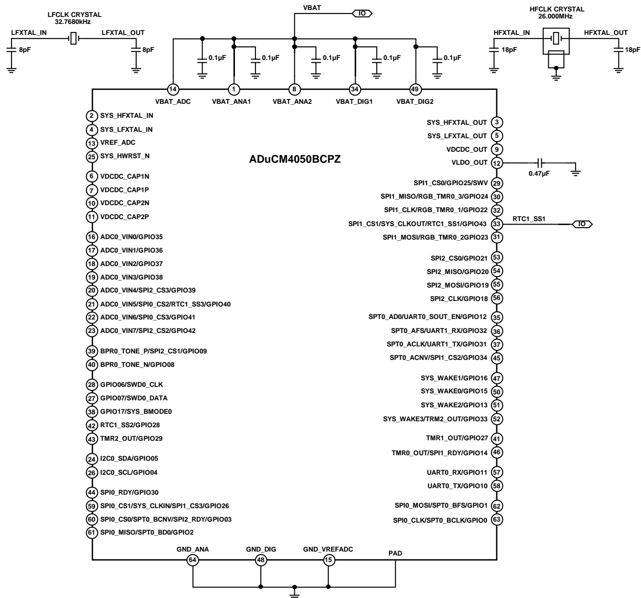
Figure 27. Recommended External Components when Using LFXTAL and HFXTAL
