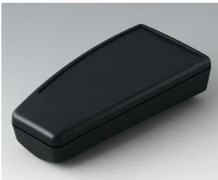
A9066319 SMART-CASE M, Vers. VI ABS (UL 94 HB) black RAL 9005 3.78"x1.85"x0.94" IP 40
