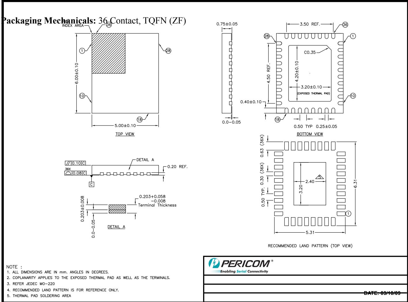
**DESCRIPTION: 36-contact, Very Thin Fine Pitch Quad Flat No-Lead (TQFN)**
