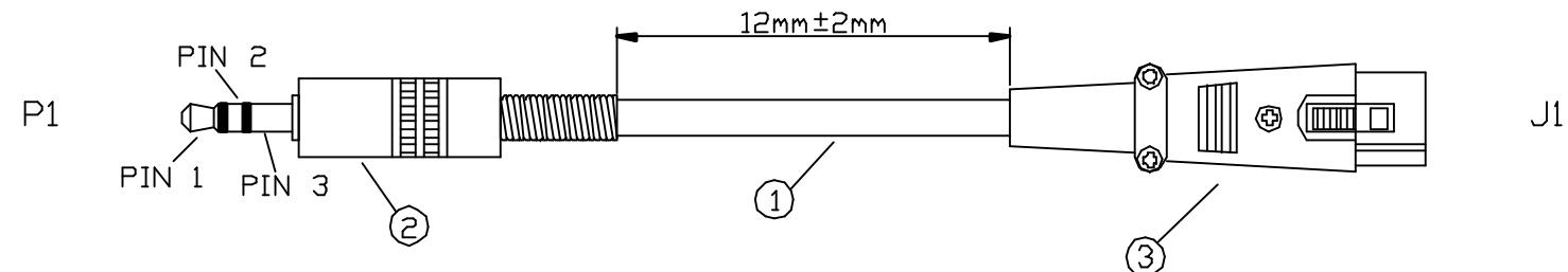
2.CONNECTOR:1 SETS 3.5mm STEREO MALE WITH ASSEMBLY TYPE
