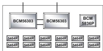
The BCM56303 is the fifth generation of the highly-integrated and cost-effective Broadcom StrataSwitch and StrataXGS product line in a single-chip solution with 24 GbE ports and three 10-GbE/HiGig+ uplink ports. The BCM56303 is a member of the Value GbE product line, with a corresponding pin compatible member in the Feature GbE product line—BCM56503. The BCM56303 incorporates 24 GbE ports that can operate 10/100/1000 Mbps. The uplink ports can operate in two modes:
