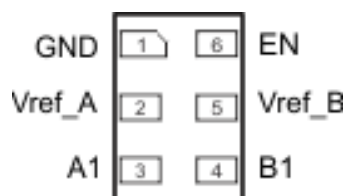
Figure 5-1. LSF0101 DRY Package, 6-Pin SON (Transparent Top View)
