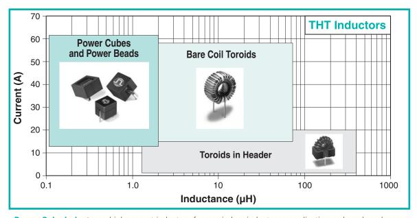
**Power Cube Inductors** - high-current inductors for use in low inductance applications where board space and height are critical
