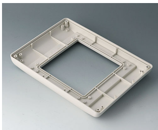
B4044707 Bottom part M flat, version I ABS (UL 94 HB) off-white RAL 9002 8.86"x6.50"x1.00" IP 54 opt.
