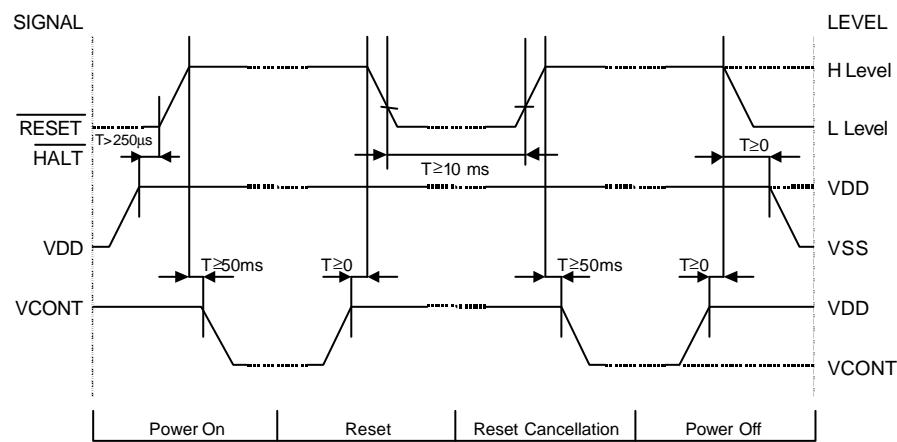
Please maintain the above sequence when turning on and off the power supply of the module.
