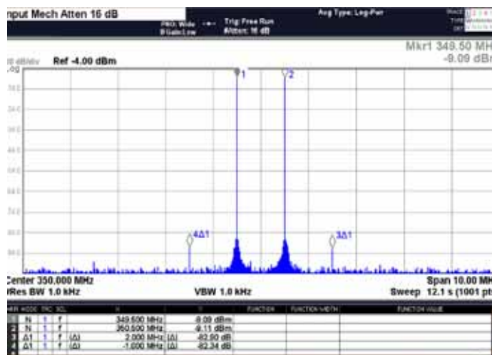
Fig 11. IMD3 (dBc) for two tones (spacing 1 MHz) centered at 350 MHz
