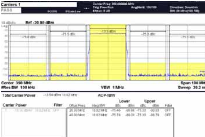
Fig 21. ACLR of 1 carrier LTE (BW=20 MHz) centered at 350 MHz
