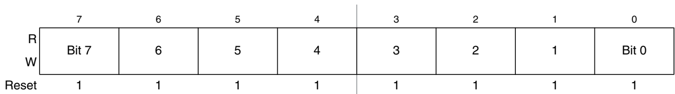
Figure 12-28. PWM Channel Duty Registers (PWMDTY1)
