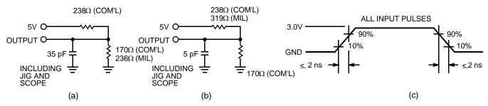
THÉVENIN EQUIVALENT Equivalent to: 99 $\Omega$  (COM'L) 2.08V(COM'L) OUTPUT O-
