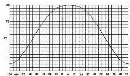
Flux Characteristics @ 350mA, T<sub>j</sub>=25°C
