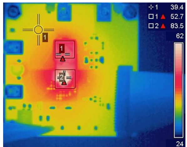
Figure 19: Thermal Image at V_{IN} = 16V , I_{OUT} = 10A (IR3865: 84^\circ C , Inductor: 53^\circ C , PCB: 39^\circ C )
