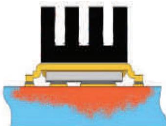
⑨ Mounted to a PCB with small clip heatsink (still air)
