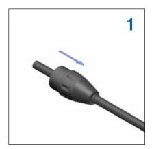
Slide the nut (Backshell) onto the cable
