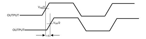
Input - Output Propagation Delay
