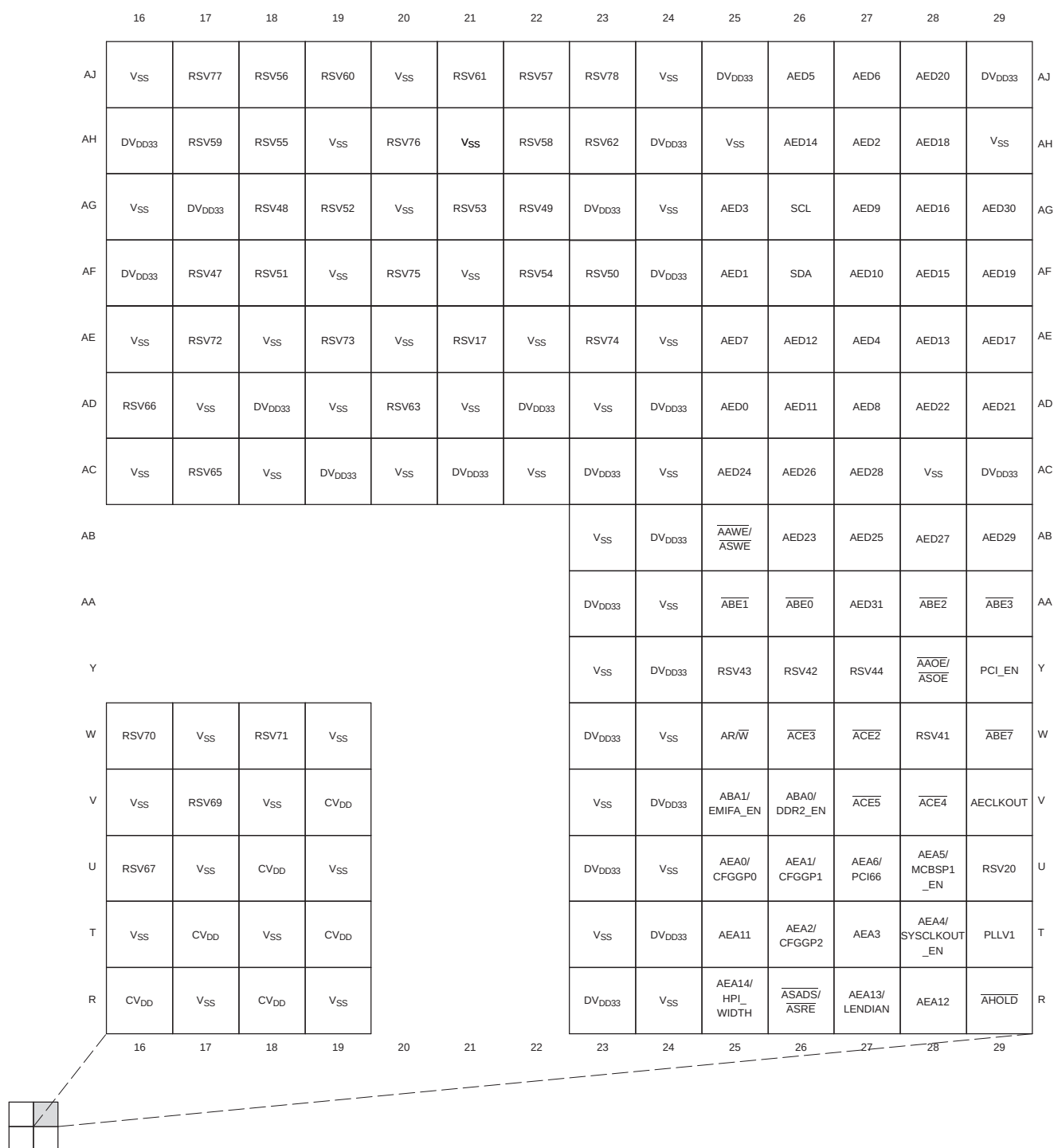
Figure 2-3. C6454 Pin Map (Bottom View) [Quadrant B]
