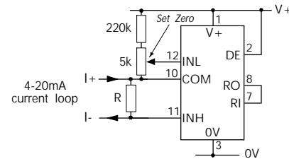
Measuring a 4-20mA loop current.
