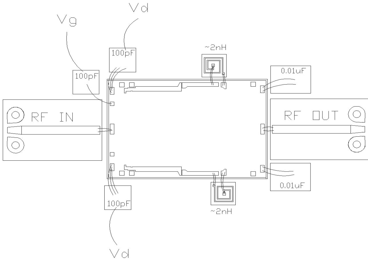
1uF or larger capacitors (not shown) should be on the gate and drain line.
