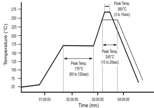
4 - Wave Soldering Process
